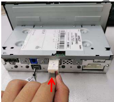
Replace the OE conversion wire with supply wire.
