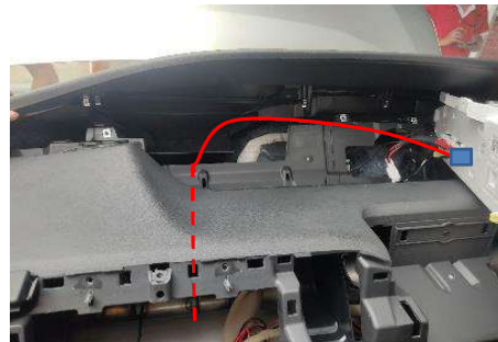
Route the T-joint wire to the radio head unit.
